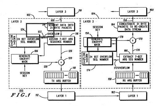
The transmit overflow sequence number 124 (highlighted in green) used in the transmitter 102 is distinct from the receive overflow sequence number 174 (highlighted in red) used in the receiver 104. Rather than use a single "overflow sequence number," the specification consistently uses the term "transmit overflow sequence number" to refer to
