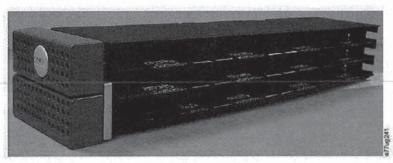
Each of the twelve slots can contain one tape cartridge, a media element, and the lower slot is a mail slot.
