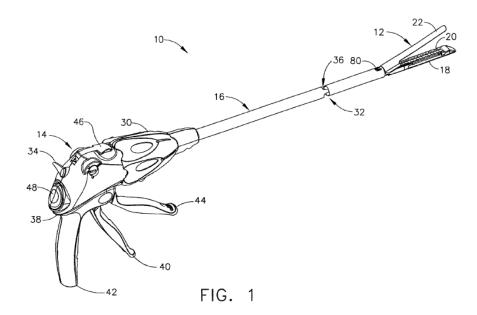
*Id.* at Fig. 1, 3:44-46 (showing a "perspective view of an endoscopic surgical stapling instruments for surgical stapling and severing in an open, unarticulated state.").
