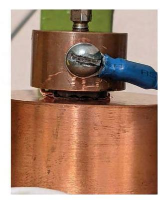
RX-0567; *see* Tr. (Bellin) at 996:6-999:12; RDX-0004C.47-.49. The soft copper pistons were pressed against the diamond table to ensure full contact across the entire top and bottom surfaces. *See* Tr. (Bellin) at 996:6-997:8. The result, which was calculated by dividing one by the resistivity and applying a conversion factor to get units of S/m, was almost four orders of magnitude less than 1200. *See id.* at 997:9-24, 999:13-1000:1.
