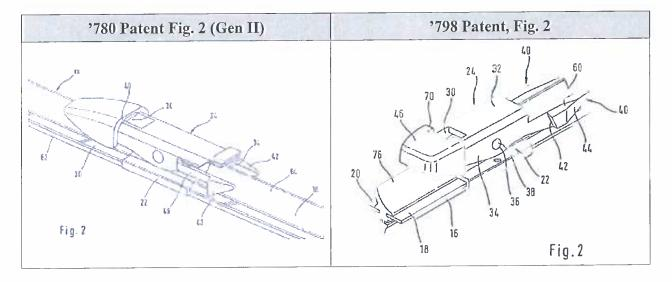
Indeed, to establish anticipation, Trico must still prove, by clear and convincing evidence, that the Gen II connector satisfies each element of the Asserted Claims. For example, Trico must demonstrate that the Gen II connector is capable of pivoting with respect to the wiper arm until a secure connection is achieved, as required by claim elements 1[h] of the '798 patent and 1[k] and 32[d] of the '044 patent. Trico suggests that such functional claim language is irrelevant. (See
